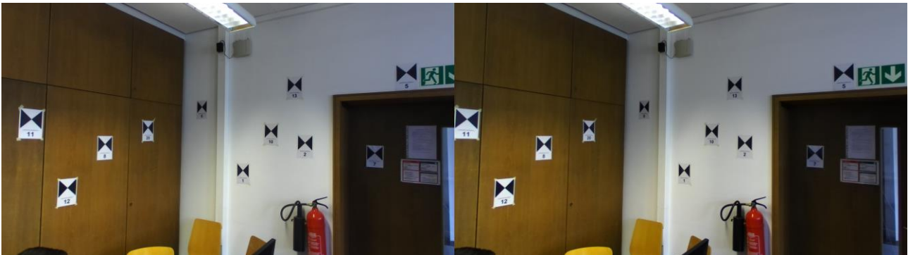
Fig. 8: left and right image of a stereo pair of the ZED camera. Control points included. One can see that the corner of the room is left of the installation channel.
