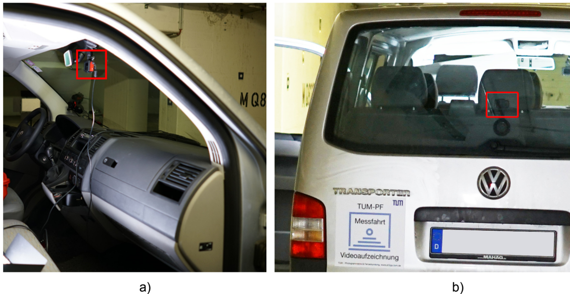
Fig. 4: a) Position (red rectangle) of the front camera, looking through the windshield to the area in front of the car, b) Position of the rear camera, looking through the rear window to the area behind the car. Image brightness strongly increased for better visualization.
