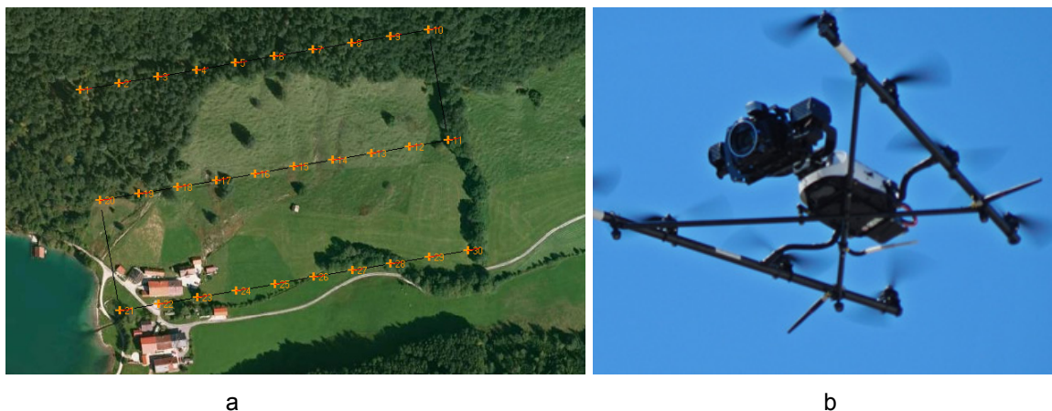
Fig. 3: a) Overview of the test site. Left is the Walchensee lake. Only the meadow areas close to the valley ground are recorded. Forest areas are skipped. b) Falcon 8 with Sony Nex 7 mounted.
