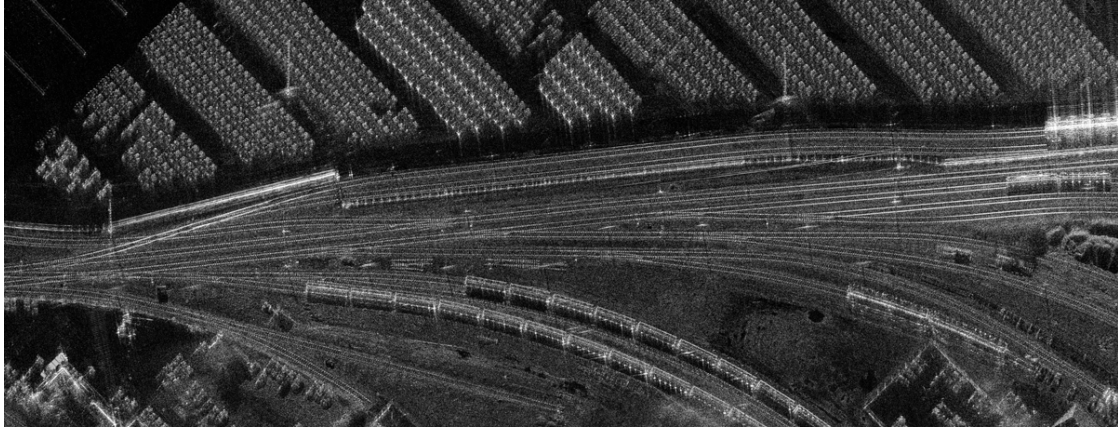
Fig. 1. SAR image of a car terminal in Bremerhaven with rail tracks, freight wagons and a fully populated parking lot.
