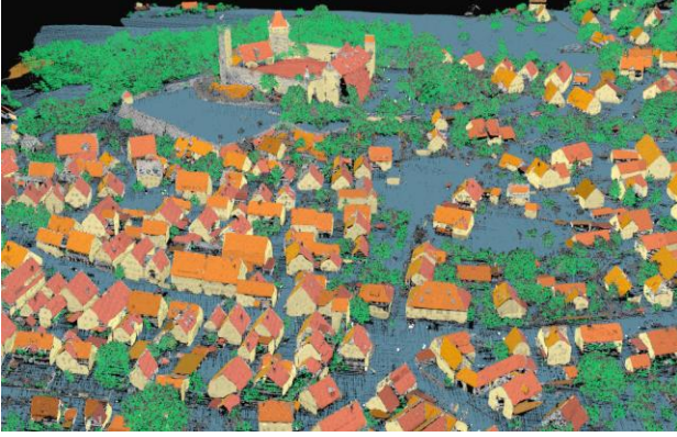
Figure 4. Partial view of the database with ground level (blue), vegetation (green) and planar patches (red).
