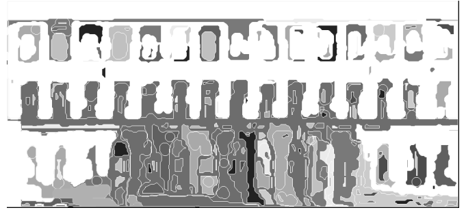
Figure 10. Region growing result. All grey parts belong to disturbing objects. Only the white parts are used in the further processing
