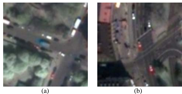
Figure 1. Spaceborne traffic scenes (Quickbird). Moving cars can be identified by their color fringe; see blue car in (a) and red cars in (b)
