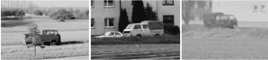
Fig. 1. Ground-based images of different vehicles (VWBUS-PICKUP). a) Scene 1: Object distance ~20m, sunny, visibility mediocre, b) Scene 2: Object distance ~130m, diffuse, clear visibility, c) Scene 3: Object distance ~320m, diffuse, dull visibility
