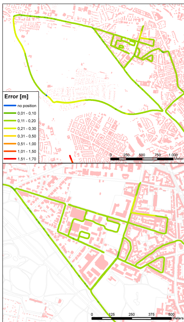
Figure 8. Map of accuracies using a precise IMU for filtering for a camera system with 100° opening angle. The accuracy along the highway (upper picture, left) depends on the direction of travel (from south to north).
