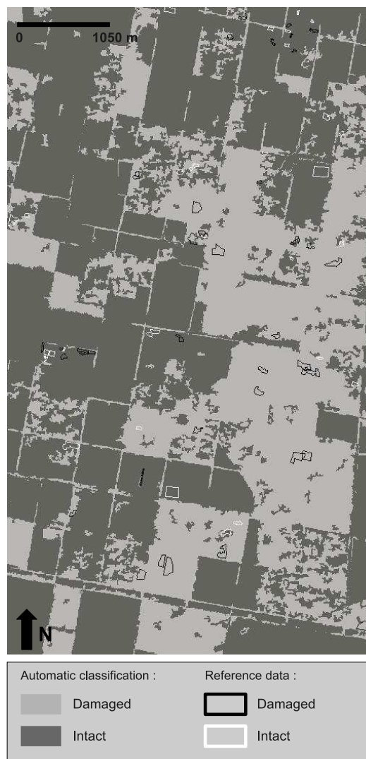
Figure 8: Binary map of wind storm damaged areas.
