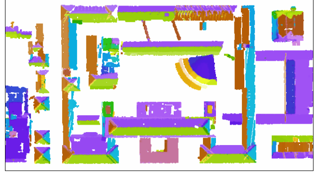
Figure 4. Remaining points after robust elimination of clutter objects, color-coded according to the normal direction
