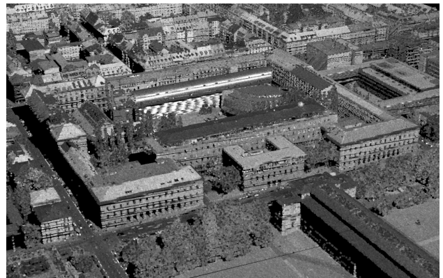
Figure 1. Laser data of an urban area scanned in 45° oblique view. Flight direction east to west (data set 4)
