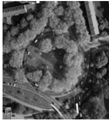
Figure 13. Example of a central island that cannot be extracted due to heavy occlusions caused by trees and shadows.
