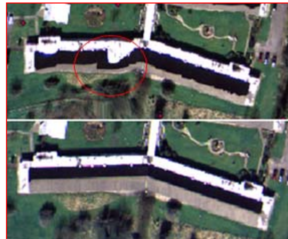
Figure 2: Effect of DSM on Building Rectification
