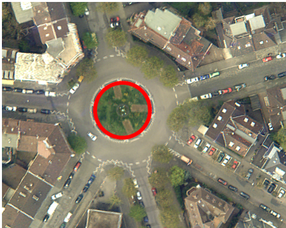
Figure 8: Hough transform applied to Mannheim dataset to find circular shapes as roundabouts
