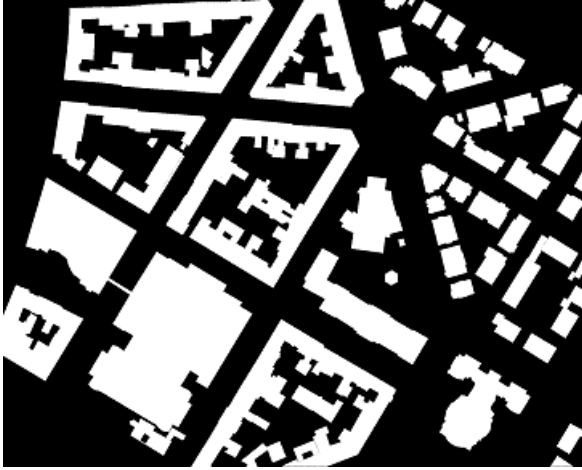
Figure 6: Ground truth used to evaluate the classification results; white pixels are buildings, blacks one are remaining objects
