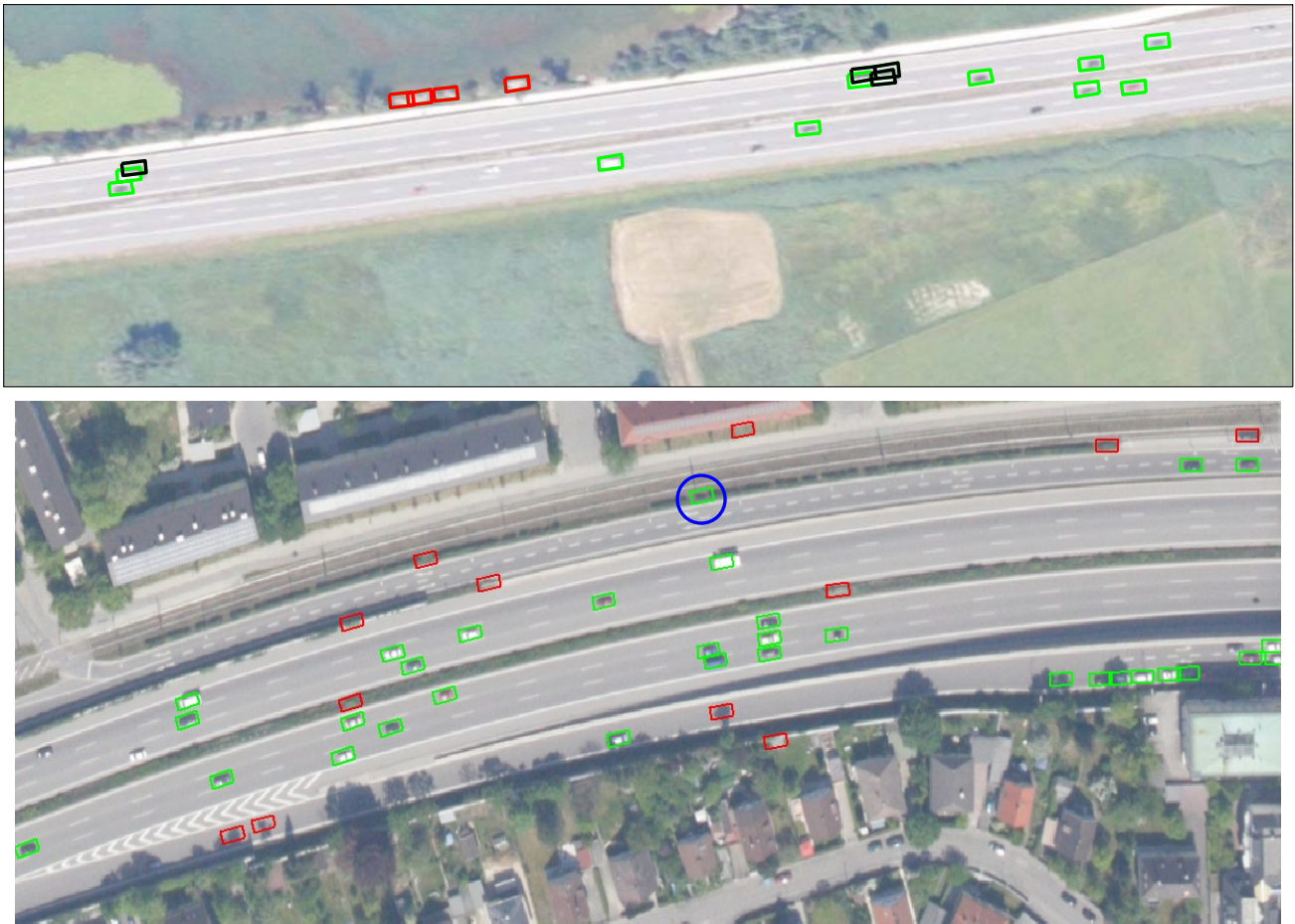
Figure 7: Results of the refinement process. Green: detected and tracked vehicles; Black: redundant objects eliminated by trajectory analysis; Red: false alarms by velocity evaluation. Blue circle: false alarm which has not been eliminated.
