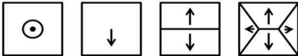
Figure 10. The face normal directions of the four basic roof shapes: flat, shed, gabled and hipped. The flat roof face shows upwards.
