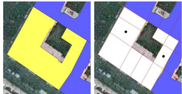
Figure 7. Cell decomposition of a given footprint into rhomboids and trapezoids, the latter marked with dots.
