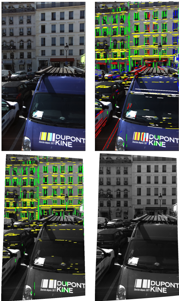
Figure 2: The rectification process. upper left: original image only; upper right: original image with segments that support main vanishing points (green and blue ones are those for the main vertical direction, yellow and white ones for the main horizontal direction and red ones for an aberrant vanishing point); bottom left: rectified image with rectified segments that support the two selected directions; bottom right: rectified image only
