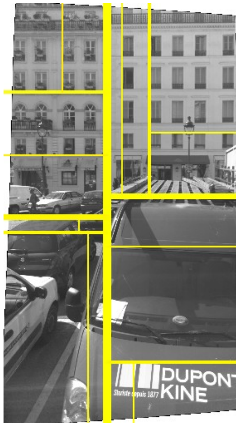
Figure 10: The process recursively segments each of the four sub-images. It splits the two façades and the foreground cars.
