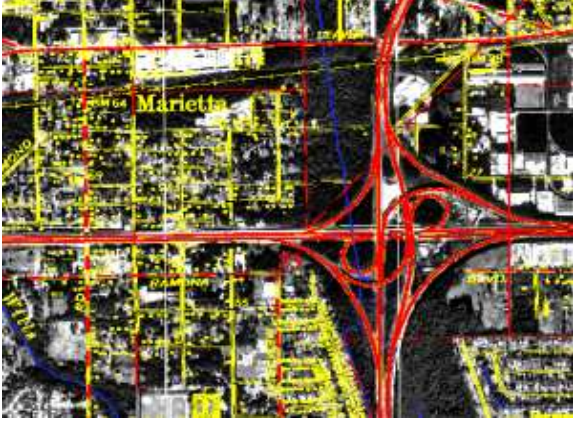
Figure 1: Map revision environment. Here previous map layers are aligned with current digital image data.
