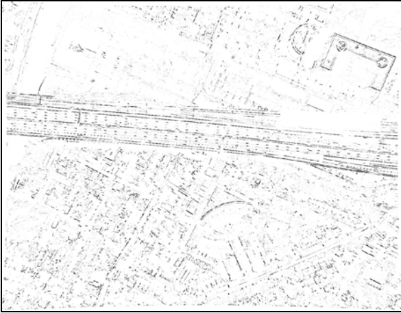
Figure 4: Line detection by morphological opening and image subtraction.
